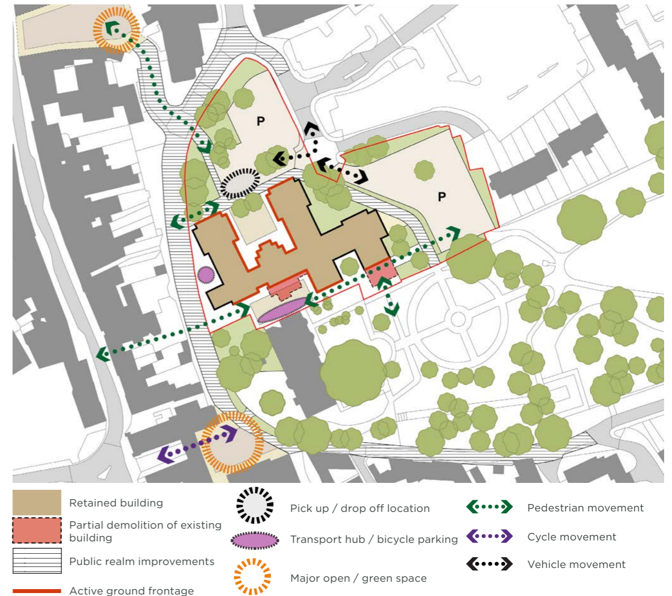
Fig 10.24: Plan setting out the key design principles for redevelopment of the Abbey House Site
